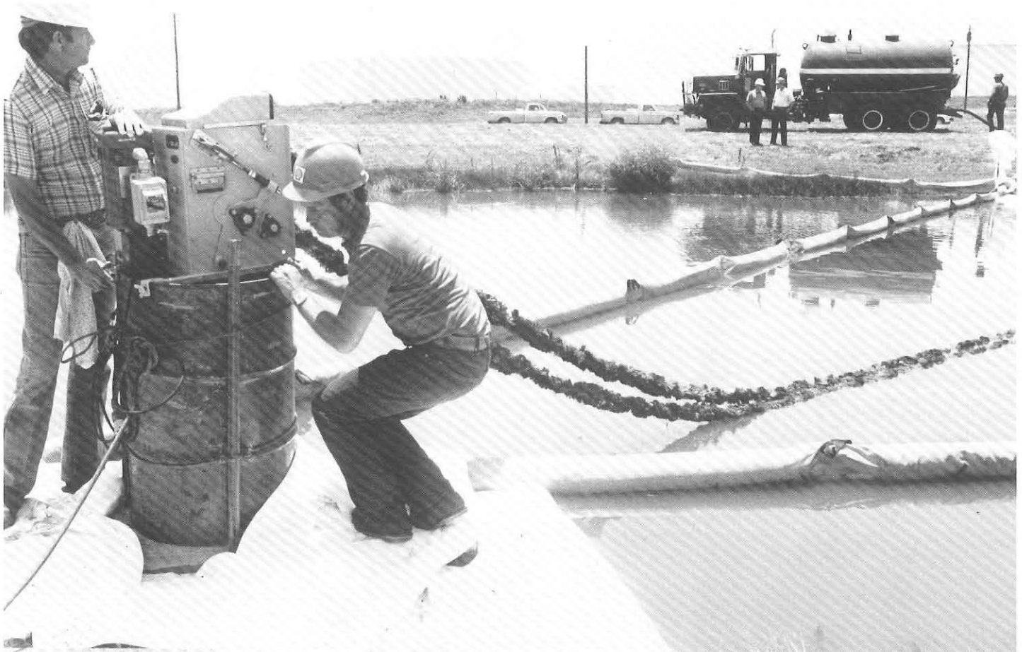
Wilson and Danny Woodcock shove the "oil mop" motor into position near the oil spill. The mop, a portable spill-absorbing machine, has only recently been introduced to Pipe Line's Oklahoma locations.
